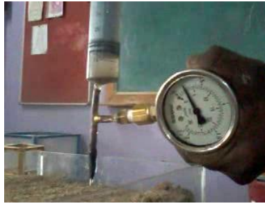
Figure.3.Injecting Grout solution in Tank
