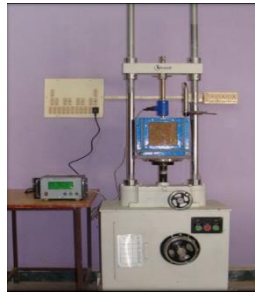
Figure.4. Triaxial Loading Frame Test
